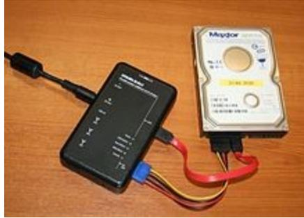
A portable Tableau write-blocker attached to a Hard Drive
