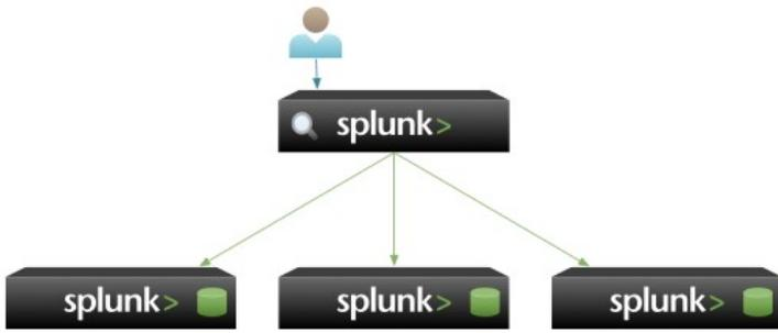
In this diagram showing a distributed search scenario for access control, a "security" department search head has visibility into all the indexing search peers. Each search peer also has the ability to search its own data. In addition, the department A search peer has access to both its data and the data of department B:
