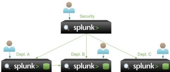
Finally, this diagram shows the use of load balancing and distributed search to provide high availability access to data:
