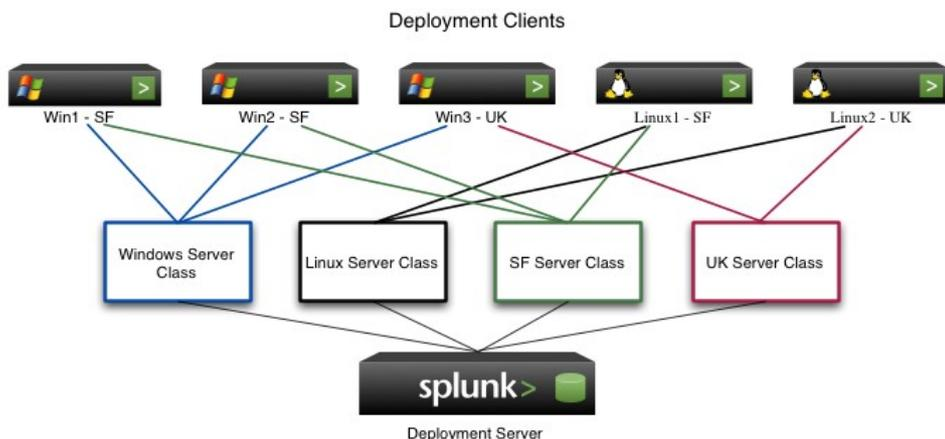
In this example, each deployment client is a Splunk forwarder that belongs to two server classes, one for its OS and the other for its geographical location. The deployment server maintains the list of server classes and uses those server classes to determine what content to forward to each client. For an example of how to implement this type of arrangement to govern the flow of content to clients, see "Deploy several standard forwarders".
