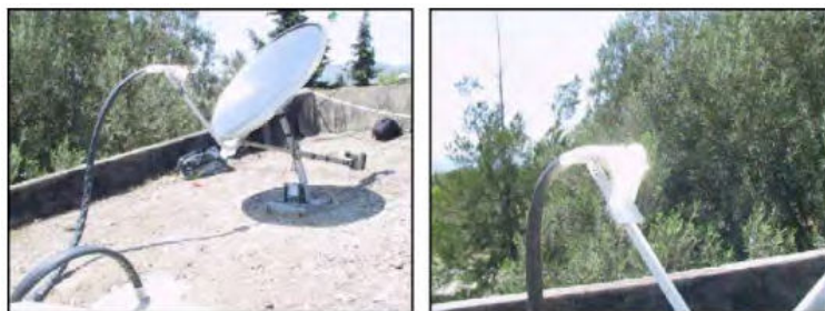
Figure 13.28 Transmission of concentrated sunlight in a fibre-optic bundle for solar lighting (Kandilli et al. , 2008).
