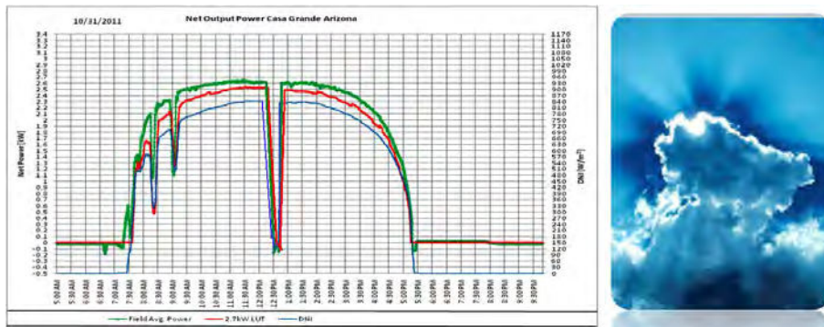
Figure 22.6 Hourly solar radiation and power generation curve for a solar receiver system operating in some overcloud conditions (Infina, 2012b).
