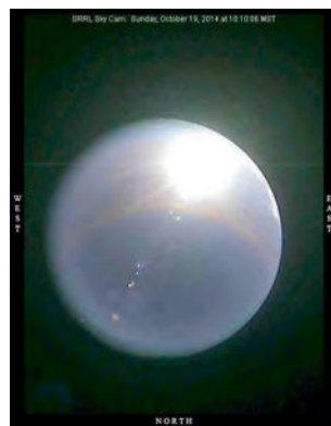
Figure 19.4 NREL solar surveying data service includes the All-Sky 180° fish eye lens as skycam webcam feature that takes images of the sun to help model the solar irradiance for a particular location (NREL, 2014a).
