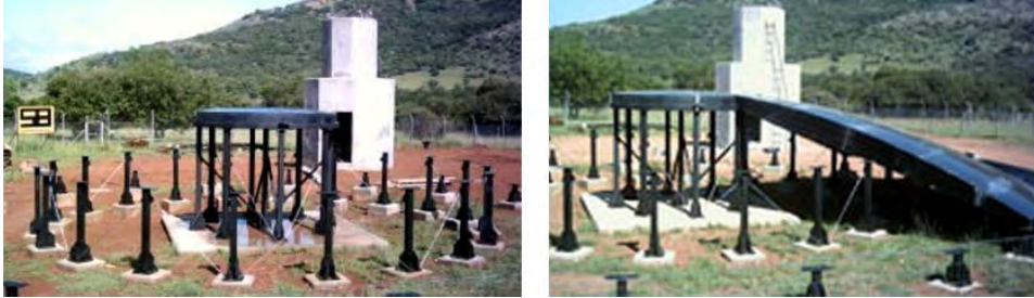
Figure 14.4 Example of a system for shaping a parabolic dish for a given diameter D size and f/D ratio in terms of upright jig pillars to shape the parabolic curve. In this example a mould is also shape to place over the pillars (image right) (SKA, 2007).
