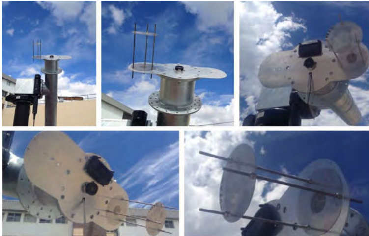
Figure 16.1 Test experiments were conducted with a test instrument and sun sensor/camera mounted onto the sun-axis of the solar concentrator boom.
