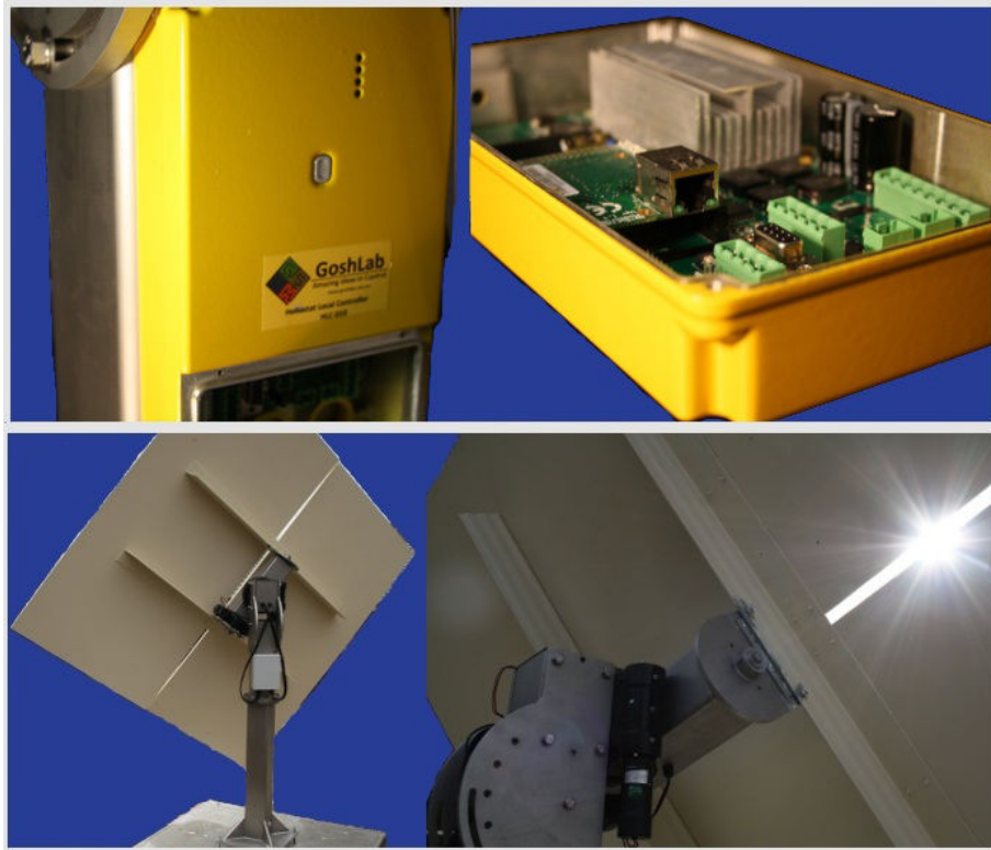
Figure 11: Goshlab sun tracking controller for concentrating solar power systems shown with a typical solar tracker system (?).
