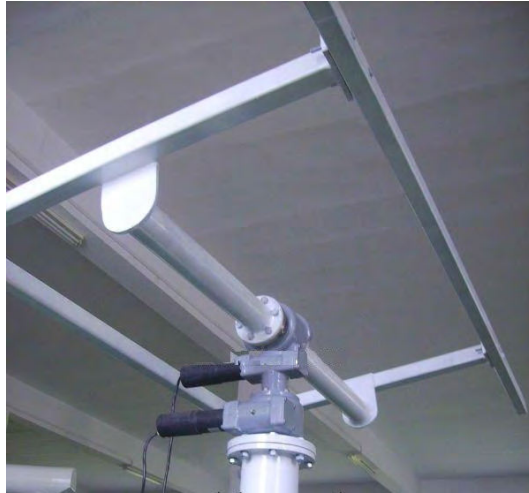
Figure 20.12 Integrated slew drive mechanism as dual axis photovoltaic solar panel tracker (BizRice, 2014).
