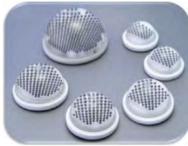
Figure 13.8 Hemispherical solar cell with collection units around all sides of a dome matrix for solar tracking (Kyosemi, 2012).
