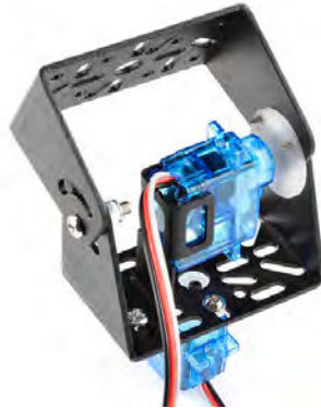
Figure 2.27 Desktop model Pan/Tilt servo platform with servo dual axis control motors (SparkFun, 2014b).
