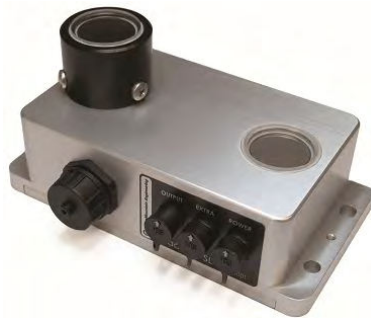
Figure 16.3 Trac-Stat SL1 a diagnostic instrument for measuring tracker accuracy (Davis and Williams, 2008).
