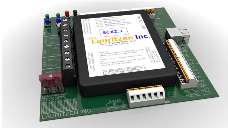
Figure 13: Lauritzen solar tracking controller (?).
