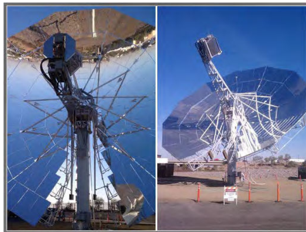
Figure 21.6 SolarCAT system of Southwest Solar, incorporating support struts for structural stability (Southwest Solar Technologies, 2013).
