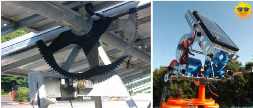
Figure 2.32 Solar tracker actuator includes a large diameter vertical gear concept (FEiNA, 2014)(Sanchez, 2012).
