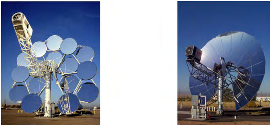
Figure 21.3 Modifications to balanced cantilever-type design of the McDonnell Douglas modular parabolic dish (WGAssociates, 2001).
