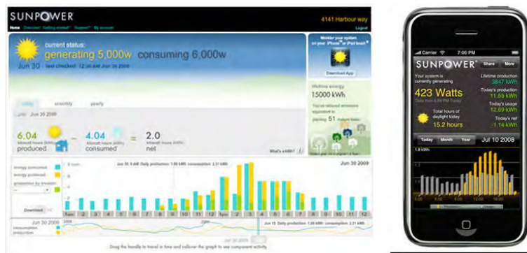
Figure 12.4 Example of solar system data acquisition and monitoring using the "SunPower Monitoring" app for mobile devices (SunPower, 2014a).
