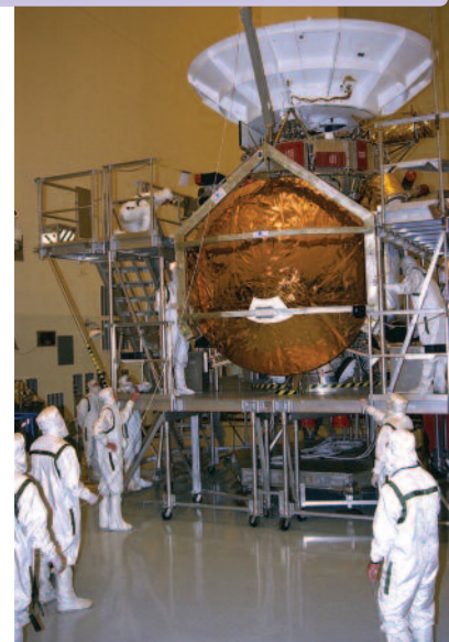
FIGURE 3: Technicians install the Huygens probe into the Cassini orbiter in July 1997.
