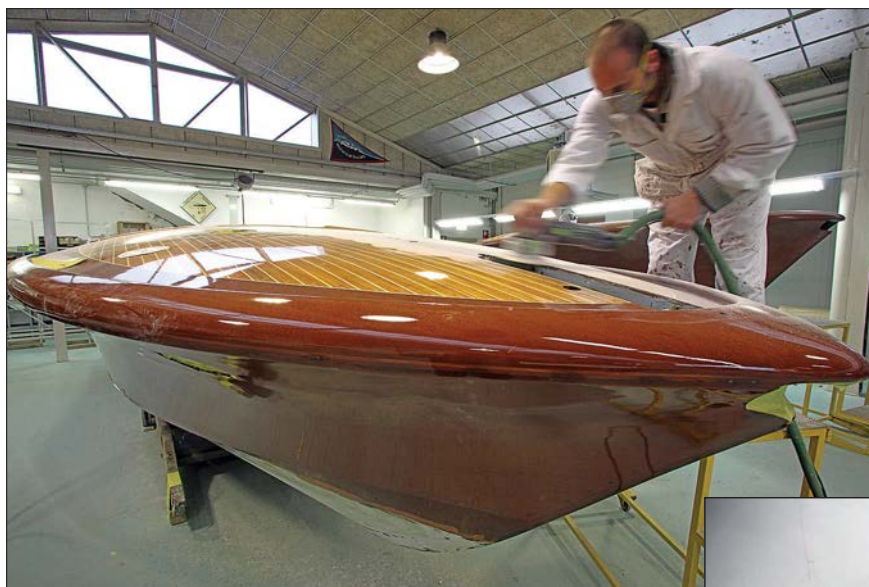
The Aquarama is the flagship model of Riva's now-discontinued line of wooden boats. Here, one of them receives a careful sanding before moving on to the spray booth for varnish.
