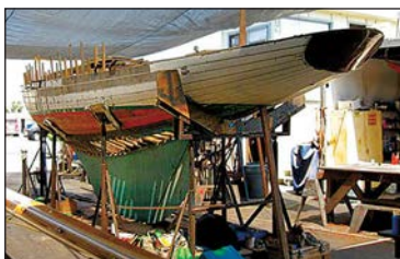
THERAPY: new floors, frames and planking
