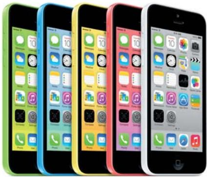
piece of plastic, and feels good to hold and well built without being heavy. The polycarbonate surface is grippy, too. It's slightly longer and a little heavier than the iPhone 5. On the inside is a A6 chip, the same processor as the iPhone 5.
