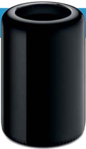
Apple has given us a 'sneak peek' of its all-new Mac Pro, which has been completely redesigned both internally and externally. The new model has a cylindrical case, and the entire top acts as a handle for carrying it. That's possible because the new version is about one-eighth of the size of the previous Mac Pro tower, and stands at 9.9in tall. The new design is built around a 'unified thermal core' that aims to keep the Mac Pro cool.
