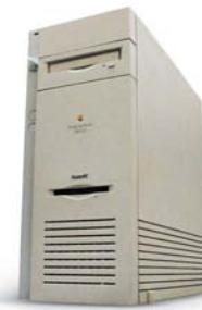
Mac based on the 9150's design.) Released in April 1994, the 9150 offered four NuBus slots and a PDS. Buyers had a choice of an 80MHz 601 PowerPC CPU or a 120MHz 601+ PowerPC processor.
