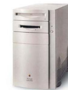
The machine had seven half-height/three full-height bays and six PCI slots, and it weighed over 35kg.
