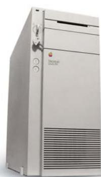
Quadra 950 (released in May 1992) had five NuBus slots, as well as a PDS. The key locked the power switch so that unauthorised people couldn't turn it on or off. The key also locked out input devices.
