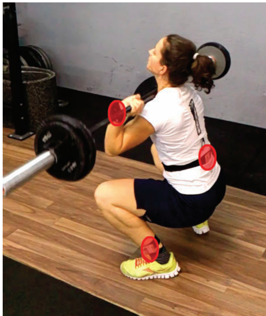
Figure 2: An athlete wearing three PIMUs in the start position of a "thruster."
