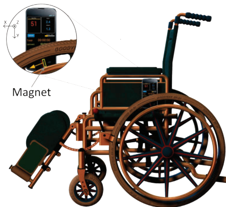
Figure 5. Smartphone instrumentation of a wheelchair.
