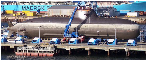
Type 212 submarine with fuel cell propulsion of the German Navy in dry dock
