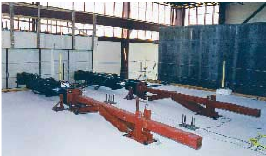
Fig. 4. Connection of actuators to floor.
