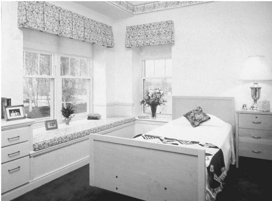
Low window seat links the bed with a view: This detail at Copper Ridge (page 201) has been popular for displaying items as well as for seating. The top is hinged for storage below. (Photo: Robert Ruschak)
