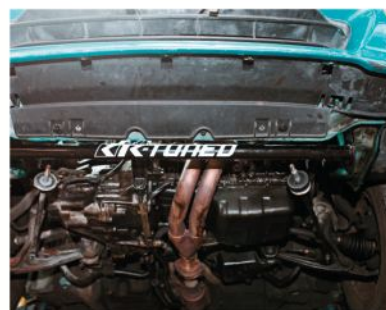
The K-Tuned traction bar is ultra solid, a direct replacement, and bolts up effortlessly.
