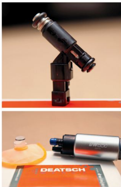
Deatschwerks set me up with a set of 600cc injectors and their ultra-quiet DW65C fuel pump. Both are E85 compatible in case I decide to make the jump.
