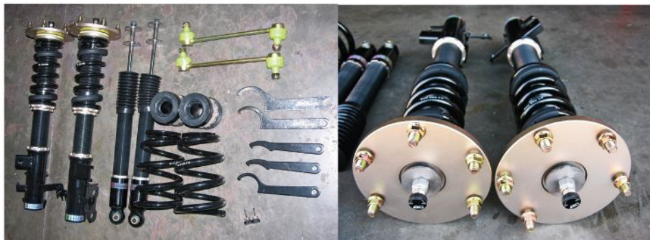
The complete BC Racing coilover kit for the RDX and a top view of the adjustment knobs and anodized finish
