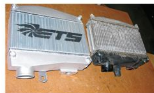
The ETS intercooler pictured here next to the anemic stock unit.
