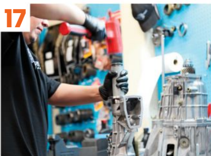
After installing the end bearing and seal, next you will drive on the companion flange onto the secondary shaft. Once that is complete a new O-ring and nut will need to be installed and torqued to 119 ft-lb. This nut will also need to be staked in place to prevent it from backing out.
