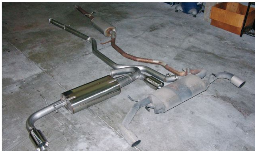
The sexy Heel-toe Automotive ATLP exhaust system next to the restrictive stock unit
