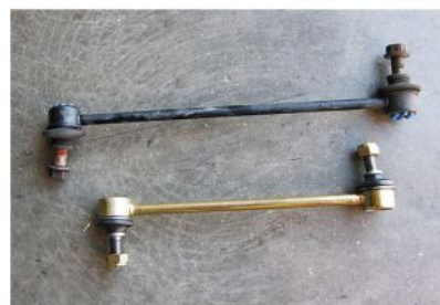
BC Racing coilovers next to the stock legs. The BC kit also includes new front sway bar end links to accommodate the thicker suspension set up.
