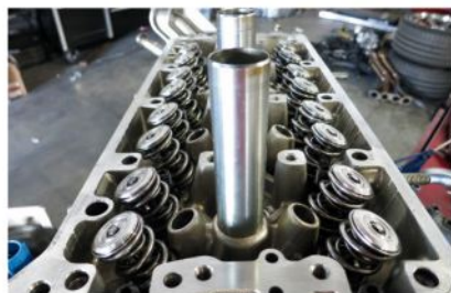
The top end was previously upgraded thanks to Supertech's tried and true valve springs and retainers. The intake and exhaust ports remain untouched.
