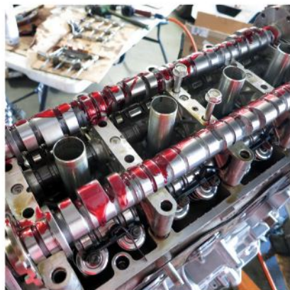
Kelford 179-B cams were chosen to keep pace with the newfound compression and they delivered ... big time.
