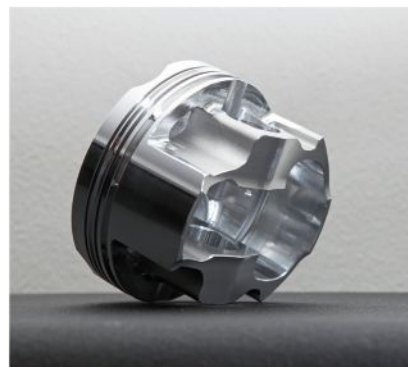
JE Pistons made quick work of producing this set of custom 87.5mm, 12.5:1 compression K24 pistons.
