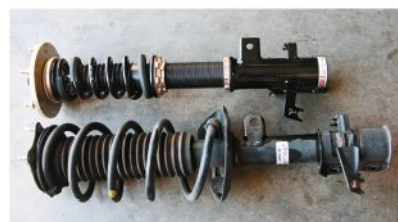
BC Racing coilovers next to the stock legs. The BC kit also includes new front sway bar end links to accommodate the thicker suspension set up.
