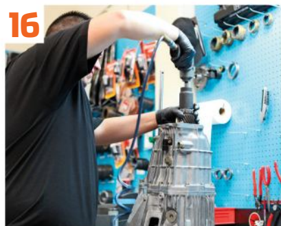
Install the secondary drive gear and bearing using a driver, then torque to 127 ft-lb. You will need a main shaft holder for the portion to keep the shafts from spinning when torquing the nut. This nut will also need to be staked to keep from backing out.
