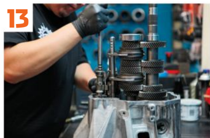
Next the shift rod is installed into the interlock and shift arm assembly. Be sure to use a new spring pin.
