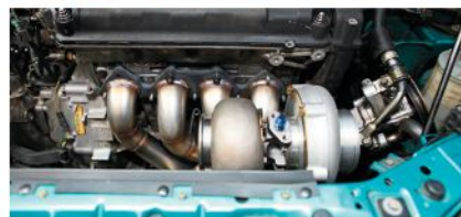
Whitfield Racing's B-series exhaust manifold. A few changes will be made in order to clearance the turbo properly. Once complete, the '90-'93 Integra manifold will be available to the public via Whitfield's website.
