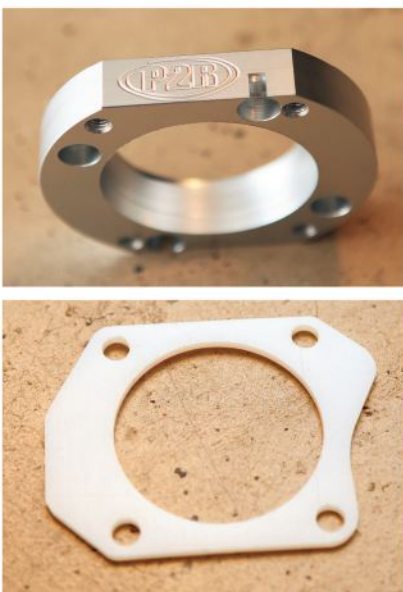
Power Rev Racing [P2R] offers a number of solutions to the cross-chassis throttle body/intake manifold dilemma. Their billet adapter and thermal gasket allowed the J35 throttle body to bolt up to the Skunk2 manifold perfectly.
