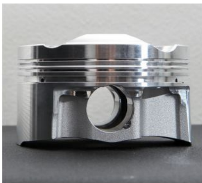
JE Pistons made quick work of producing this set of custom 87.5mm, 12.5:1 compression K24 pistons.
