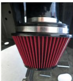
Hybrid Racing's 3.5in cold-air intake brings in even more fresh air with its 6in velocity stack and high flow filter.
