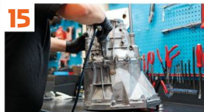
Put a nice bead of Hondabond onto the clutch housing case sealing surface and allow it to tack up for a few minutes before installing the main case. These 8mm bolts will be torqued to 20 ft-lb.
