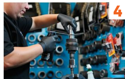
Needle bearings and distance collars are well oiled during assembly using Honda MTF. This is a crucial step to avoid a dry start up
