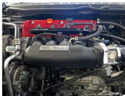
A Skunk2 Pro Series intake manifold replaces the original RBC with a larger plenum and short, slightly larger runners.
