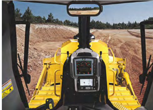
Aligning the precleaner, exhaust stack, single lift cylinder and grade-control mast with the D7E's single, center cab post provides the clearest view a dozer operator will find.
