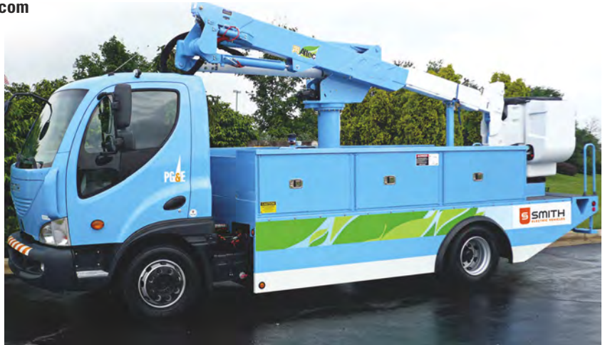
The battery-electric Smith Newton, proven in other applications in England, is being tested in California with a 38-foot aerial work platform.
