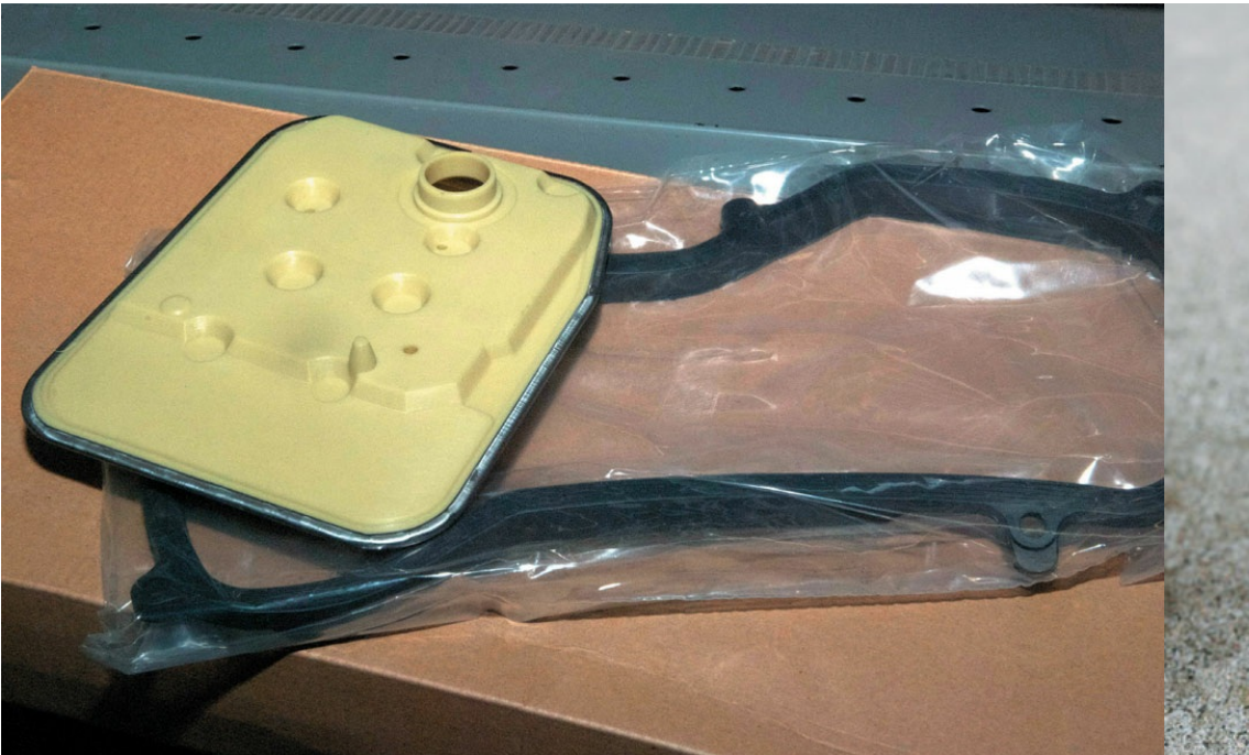
A typical transmission filter: Transmission fluid is nothing more than hydraulic oil designed to produce internal hydraulic pressure and cool and lubricate the unit. Transmissions by their very nature produce wear material that has to be filtered out of the fluid. This is the job of the transmission filter. Whenever a transmission service is done, use an OEM-quality filter to ensure maximum filtration. Transmission filters take various shapes to fit the pan configuration of a particular transmission.
