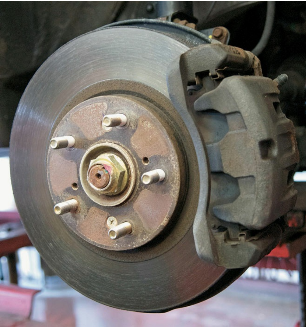
This photo illustrates a brake caliper and how it is mounted on a vehicle. Note how it straddles the disc (or rotor) with the pads sitting on either side of the disc. When hydraulic pressure is applied to the caliper, it squeezes the pads tightly together, creating friction against the disc and thus stopping the rotation of the disc, which is attached to the wheels.
