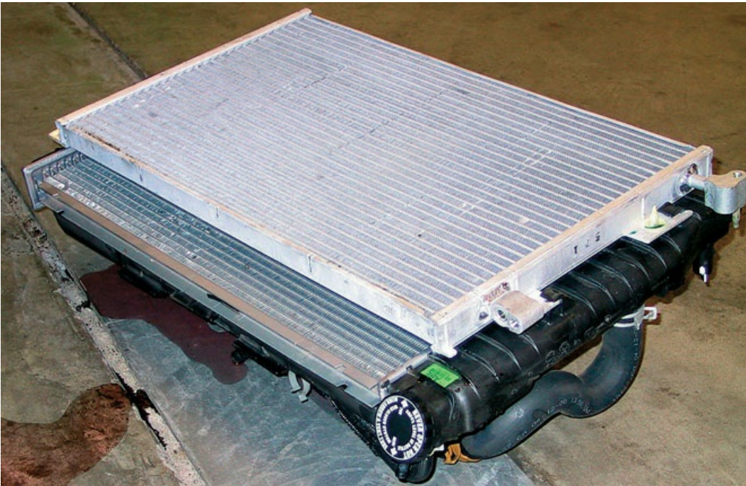
Automotive radiators vary in shapes, sizes, and what they are made of. Radiators of old were made of tin; today's radiators are made of aluminum and plastic to save weight. The shape and size depends on cooling system capacity necessary to cool the engine and body design. You can get special radiators that provide greater cooling ability for special applications like towing, racing, or off-road applications.
