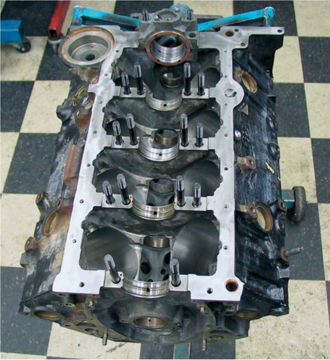
The engine block is cast of aluminum or iron. All the necessary holes for internal components such as pistons, camshafts, valve lifters, and bearings are cast into it. In addition, oil galleries for lubrication, water jackets for internal cooling, and mountings for external components are cast into the engine block.
