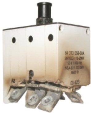
Overheated 50Amp CB
