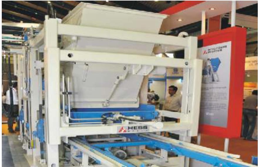
Latest generation machines can churn out thousands of blocks in a variety of sizes and shapes
