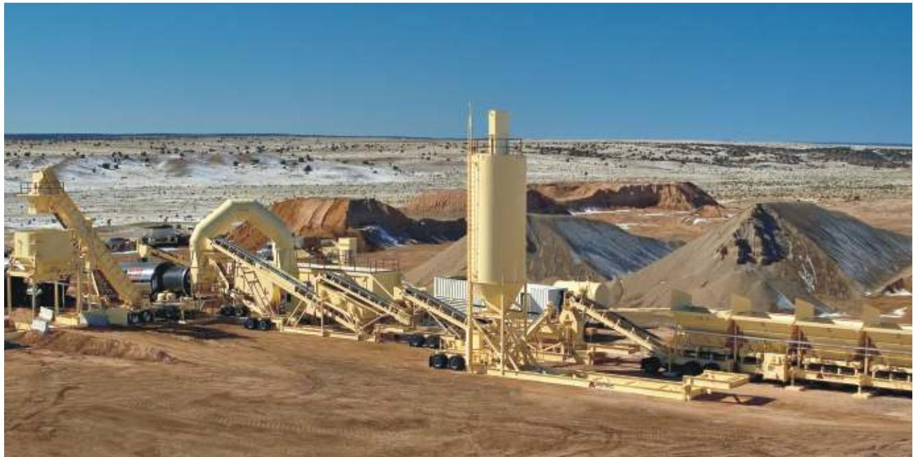
TIL- ASTEC double barrel hot mix asphalt plant
