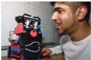
In this third year project the student built a robotic face (from Lego mindstorm) capable of expressing emotion, and software that allowed the robot to respond to the tone of the user voice. In the future many more devices around the home may have the ability to recognise and respond to emotion. [\[Watch the video\]](#)
