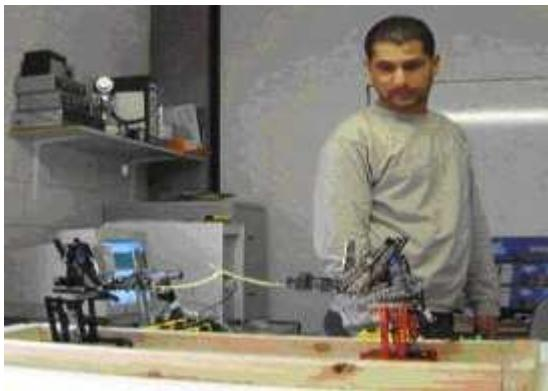
This project involved the building of two robots who fenced with each other. One robot was controlled by a flexible exoskeleton that the student built to convert his arm movements into movements in the robot. The second robot was controlled by artificial intelligence: its skills in fencing were created by obtaining 'know how' from experts on the college Fencing team and building a set of rules for the robot to follow allowing it to react to the attacking robot in a human like way.
